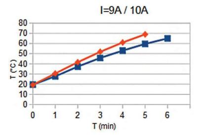
Temperature versus time with 9 A (blue) and 10A (red) current per pin, all pins loaded. (225 / 250A in total)
